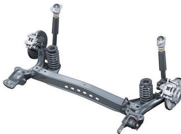
Abb.2: Verbundlenker-Hinterachse Fig. 2: Twist beam rear axle
